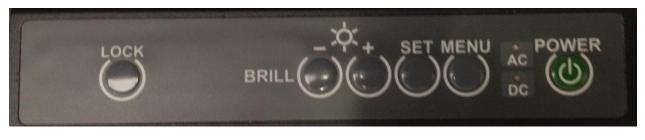
Figure 2. Front Panel with controls and indicators.
